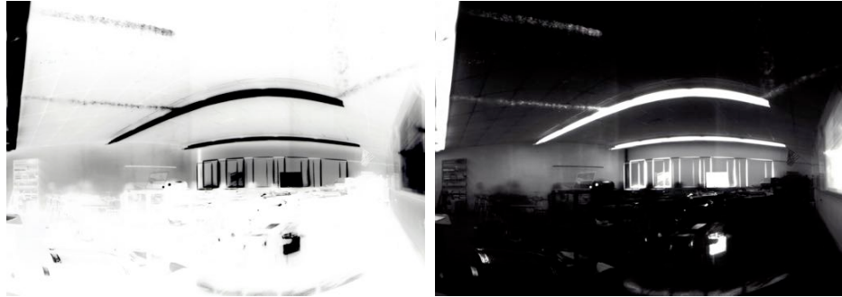
Figure 6 – (Left) Pinhole photo taken with a cylindrical oatmeal box camera, 30-minute classroom exposure. (Right) Inverted image.
