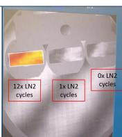
Zygo measurements for the different stressed samples were < 1/10 wave
