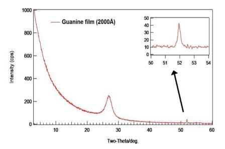
Figure 9. X-ray diffraction of physical vapor deposited guanine powder on SiO<sub>2</sub>/Si substrate.
