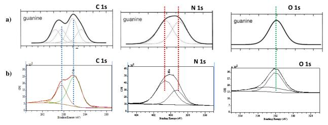
Figure 6. X-ray photoelectron spectroscopy of guanine a) guanine crystal measured by S. Ptasinska, A. Stypczynska, T. Nixon, N. Mason, D. Klyachko & L. Sanche, "X-Ray Induced Damage in DNA Monitored by X-Ray Photoelectron Spectroscopy, *Journal of Chemical Physics*, **129**, 065102, (2008) and b) physical vapor deposited guanine powder.
