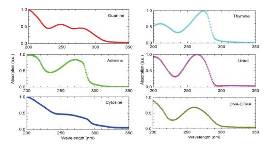
Figure 7. Absorption spectra of molecular beam deposited nucleobases.
