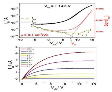
Figure 2. Transfer & output characteristics of C<sub>60</sub> OFET with 300 nm thick, "DNA-like" sequence gate dielectric, GTAGCGAGC: (G: guanine; T: thymine; A: adenine; & C: cytosine), operating voltage 15 V (due to high surface roughness), capacitance per unit area  $C_{0d} = 10.2 \text{ nF cm}^2$ , field-effect mobility  $\mu = 0.1 \text{ cm}^2/\text{Vs}$  [5, 6].
