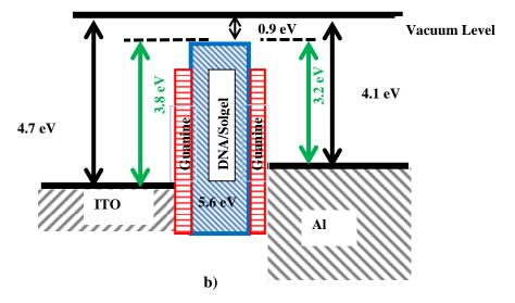
Figure 11. Layout of a) ITO/DNA-CTMA -sol-gel/Al capacitor structure and b) layered ITO/guanine/DNA-CTMA-sol-gel/guanine/Al capacitor structure.
