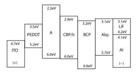
Figure 12. OLED structure.
