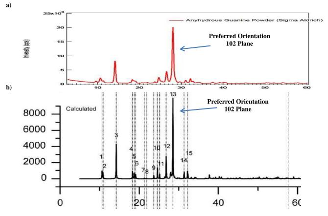
Figure 8. a) Measured and b) theoretical x-ray diffraction pattern of anhydrous guanine.
