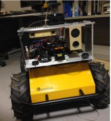
Figure 5: Fully configured research platform. Top shelf: bumblebee stereo (left), GDRS uLadar (center), ADONIS (right). Bottom shelf: gps (left), hokuyo Ladar (center), teleop receiver (right).
