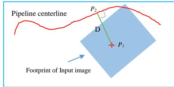
Figure 8: Demonstration of the distance calculation method.
