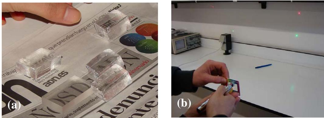
Fig. 5. Experiments to demonstrate (a) birefringence using calcite crystal and (b) diffraction from grating.
