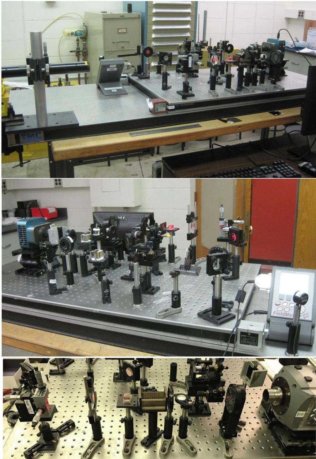
Figure 12. Experimental setup for single-photon interference lab at different viewing angles. TOP: The whole view including a He-Ne laser from a Young's double slit interferometer side; CENTER: View from a Mach-Zehnder interferometer side. A conventional CCD camera without cooling and amplification of the signal is used on top and center images. BOTTOM: A Young's double slit interferometer setup with an EM-CCD camera and a slit set with air slit opening (a He-Ne laser is not shown).
