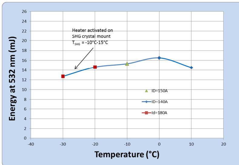
Fig. 3. Energy at 532 nm versus laser temperature
