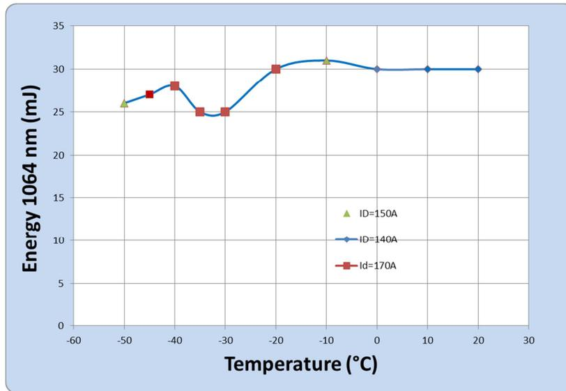
Fig. 2. Energy at 1064 nm versus laser temperature
