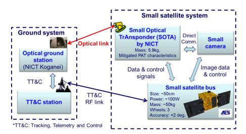
Fig. 1. Configuration of Space Optical Communications Research Advanced Technology Satellite (SOCRATES). Proc. of SPIE Vol. 10562 105624A-2
