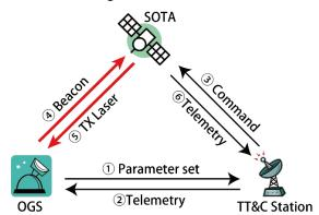
Fig. 4. Configuration of the experimental system
