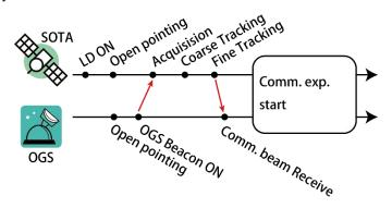
Fig. 5. Sequence of events for optical communication experiment
