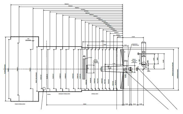
Fig. 3. CHEOPS instrument optical design including the baffling system
