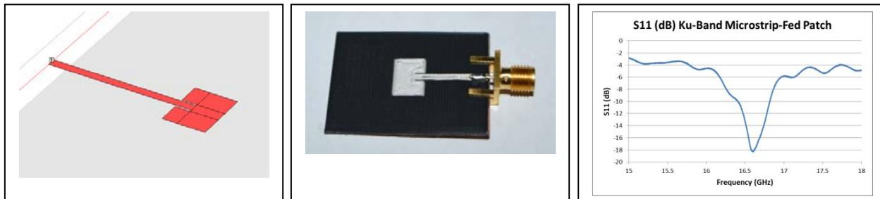
**Figure 15.** (left) Conceptual diagram of Ku-Band microstrip-fed patch antenna; (middle) actual Ku-Band antenna; (right)  $S_{11}$  characteristics of the Ku-Band microstrip-fed patch antenna
