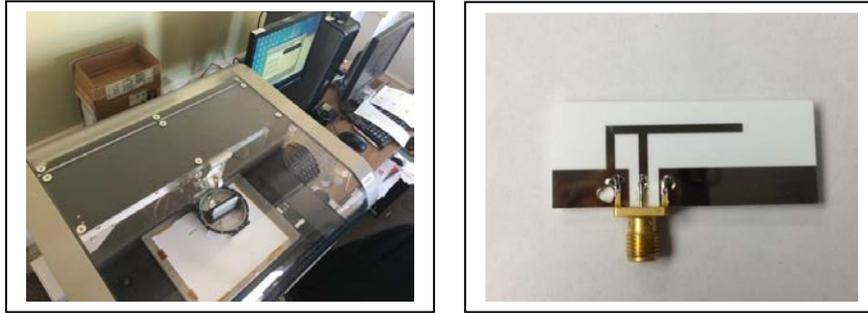
**Figure 10.** (left) Dimatix DMP-2831 Inkjet Printer and (right) Connectorized Planar Inverted F Nanoparticle Silver Antenna on Flexible Paper Substrate
