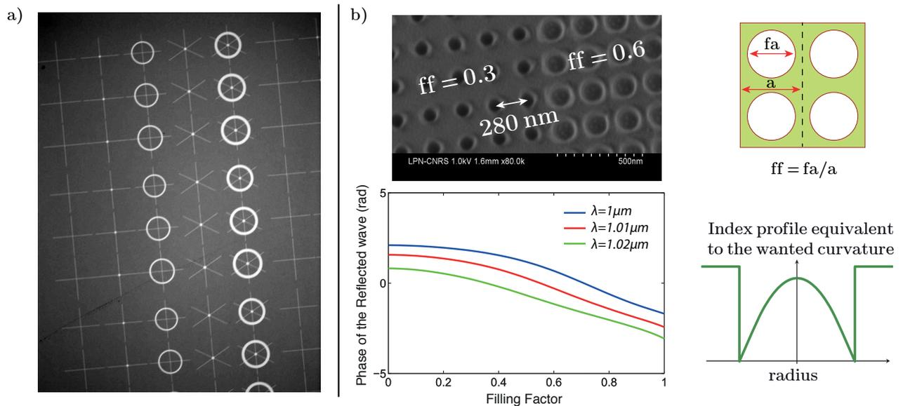
Figure 2. a) Picture of the metallic masks deposited at the surface of the 1/2 VCSEL, permitting the generation of various modes chosen in the LG base. The typical size of each pattern is  $\approx 250\mu m$ . b) Scanning electron microscope picture of the PC structure (period 280 nm) for the maximum step index. Large holes = 0.6 filling factor; small ones = 0.3. PC Phase variation curves as a function of the filling factor, and targeted phase profile for a concave mirror.
