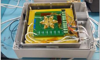
Fig. 1. Radiation testing board with the six HV optocouplers. Proc. of SPIE Vol. 10563 1056359-2
