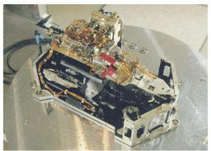
Fig. 1. The core unit of ENVISAT/MIPAS: Interferometer
