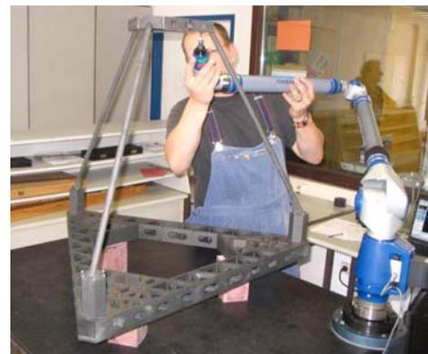
Fig.12 Integrated support structures and its 3D measurement
