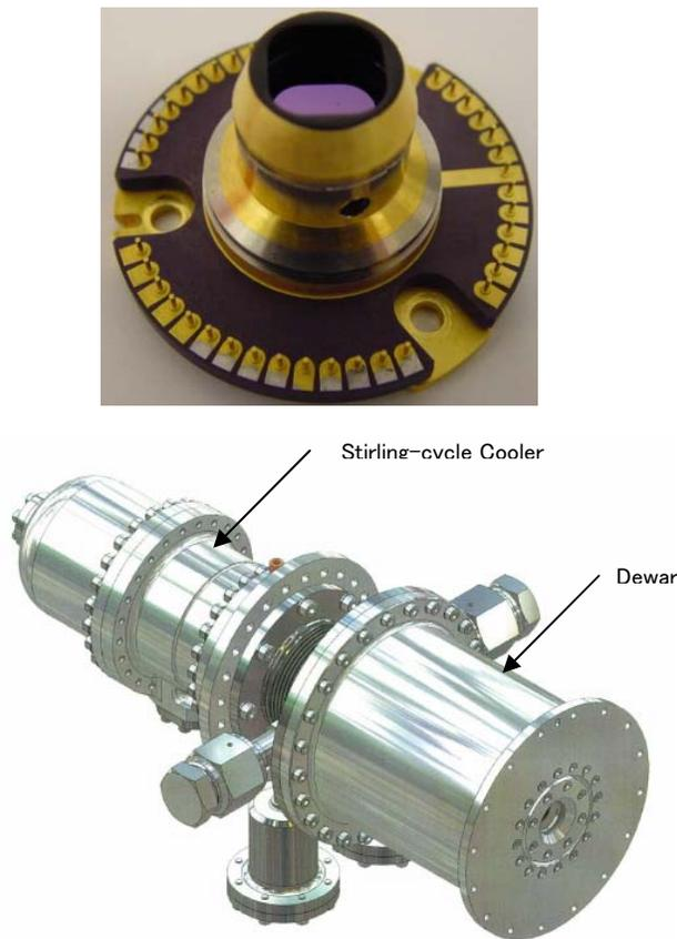
Fig. 6 TIR detectors(top) and TIR detection unit(bottom)
