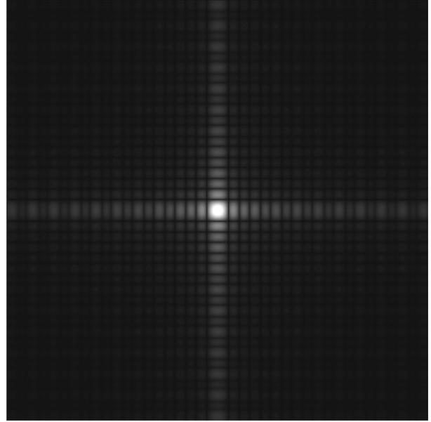
Figure 2: Example of Point Spread Function of an apodized Fresnel Diffractive Array. The brightness scale has been strongly flattened for display, to reveal the faint residual light in the four quadrants of the field.
