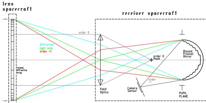
Figure 3: Synoptic diagram of an achromatized Fresnel Diffractive Imager. In the ultra-violet domain ( $\lambda < 250\text{nm}$ ), a blazed Fresnel Mirror plays the major role in the chromatism correction scheme.
