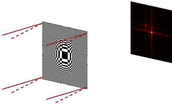
Figure 1: Image formation by a Fresnel Array. Here, a double point source is imaged by an orthogonal geometry one.
