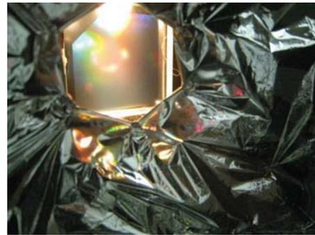
Figure 14: DCG - O2B grating - Picture of grating increase of scattering when regulation lamp is switched on.
