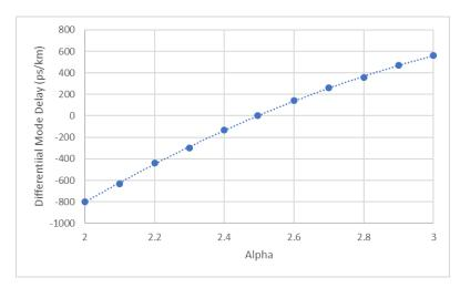
Figure 3. Differential mode delay as a function of alpha
