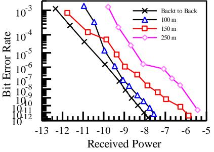
Figure 6. BER vs received optical power for the fiber with graded-index refractive index profile
