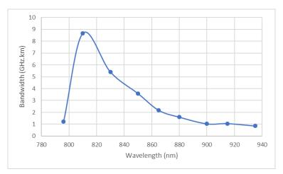
Figure 4. Measured bandwidth of graded index standard single-mode fiber.
