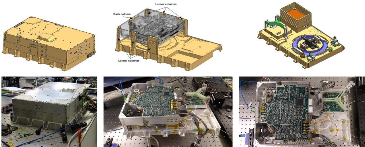
Figure 10 – Several views on the LHA 3D CAD design and the LHA EM manufacturing and integration.
