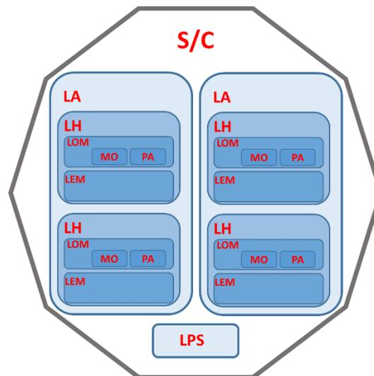
Figure 2. Laser system on board of each of LISA spacecraft. Two Laser assemblies, one for each arm, containing two Laser Heads. LH including Laser Optical Module, Laser Electronics Module. LOM composed of Master Oscillator and Power Amplifier. Frequency characteristics guaranteed by the Laser Pre-stabilisation System.
