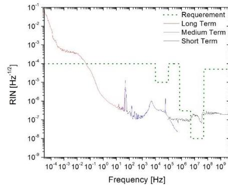
Figure 13 - RIN measurement for 1.2 W output optical power.
