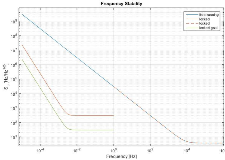
Figure 3. Laser system frequency stability characteristics free-running (blue), locked (orange), locked goal (green)
