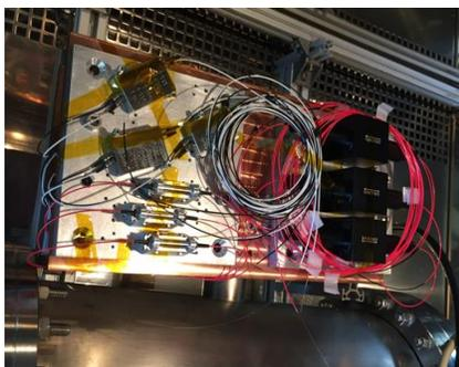
Figure 8 - Photonic devices under TVAC test.
