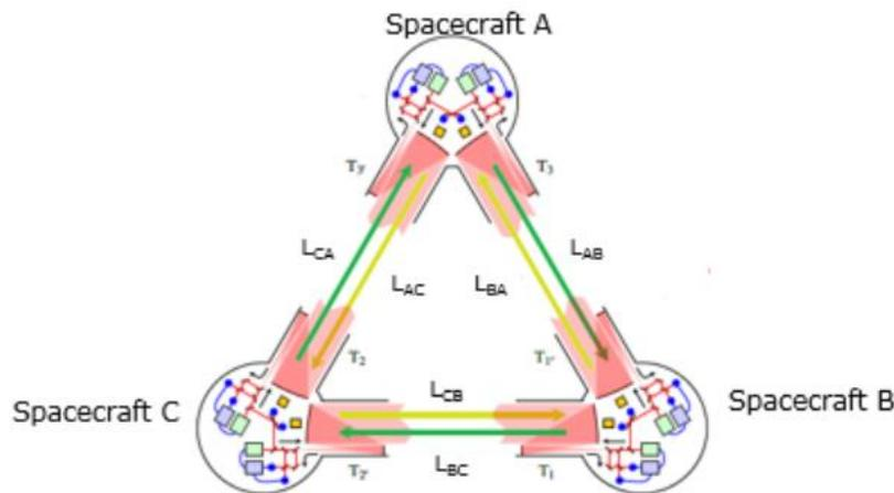
Figure 1. LISA antenna laser links. Three S/C in constellation, 3-arm interferometer, 6 1-way links.
