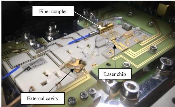
Figure 6. Micro-integrated ECDL BB with external cavity during integration.
