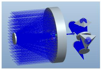
Fig.3 Optical system of thermal emission spectrometer
