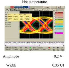
Figure 10 : Manufacturer A eye diagrams at cold and hot temperatures
