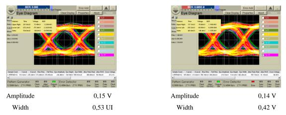
Figure 12 : Manufacturer C eye diagrams at cold and hot temperatures
