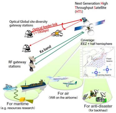
Figure. 2. Schematic drawing of the next generation High-Throughput Satellite (HTS).
