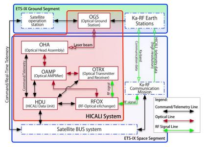
Figure 3. the functional block diagram of HICALI system.
