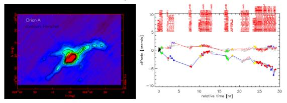
Figure 5: Left: The image shows Orion seen by PILOT and the contours are from Herschel. Right: Evolution of the pointing average offsets, cross-elevation (open circles), elevation (filled circles). In grey, the preliminary pointing model predictions.
