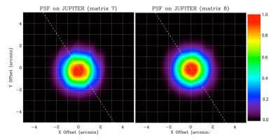
Figure 4: Point spread function of the PILOT telescope obtained during the second flight.
