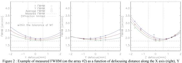
$x_1$  (right) axis (center), Z axis (left). For each axis, a defocus of 0mm corresponds to the best theoretical focus.
