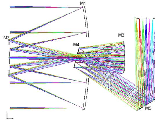
Fig. 4. WFI telescope optical design
