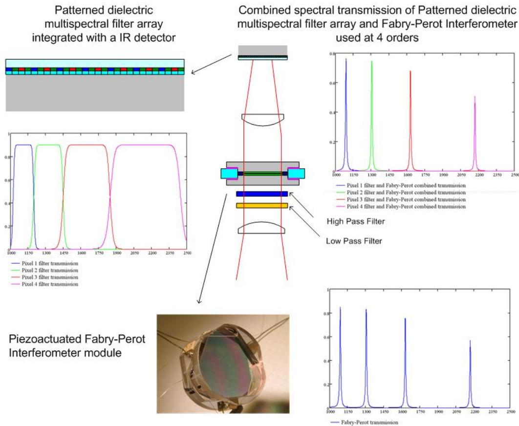
Fig. 2. Concept of the SIMACC spectrometer based on patterned multispectral pixelized filter array integrated with an IR detector. The Fabry-Perot Interferometer is used at several orders simultaneously.
