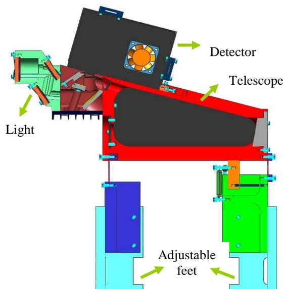
**Fig. 4.** Mechanical design for the IR optical detection system.
