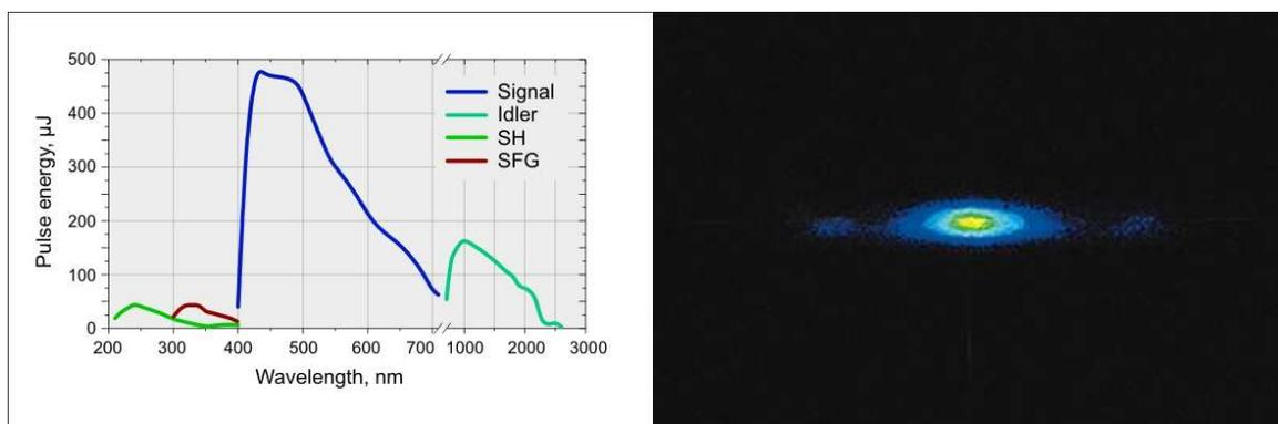
**Fig. 5.** Laser characteristics of EKSPLA NT242 OPO laser: on the left side the laser power and on the right side the beam profile as provided by the manufacturer. SPIE Vol. 10565 105656A-5
