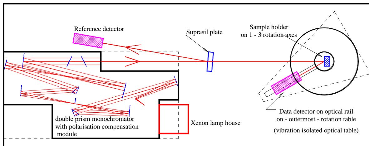
Fig. 1. Schematic drawing of the Absolute Radiometric Calibration Facility
