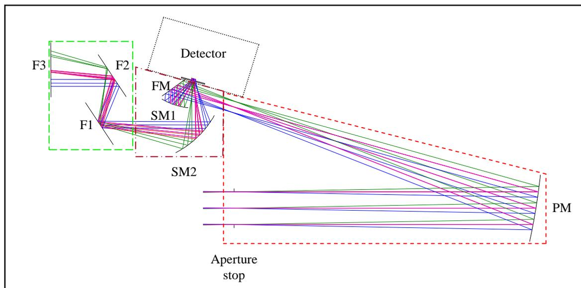
**Fig. 2.** 2D layout of the ARCF IR detector assembly with identifying components labels.
