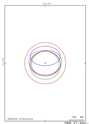
**Fig. 3.** Footprint plots at the detector of the IR ARCF configuration. The effective aperture of the detector is drawn in red. The footprint for the on-axis field is represented in black. The footprints for the full field are shown in blue, brown, green and pink.
