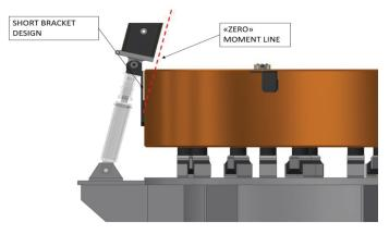
Figure 5. Gravity release mechanism for the 3 legs of the CFRP structure.
