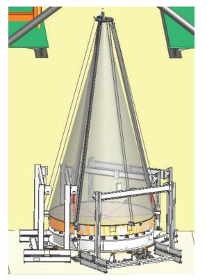
Figure 4. UV source supporting structure (above the mirror) and the 54 pads below the mirror.
