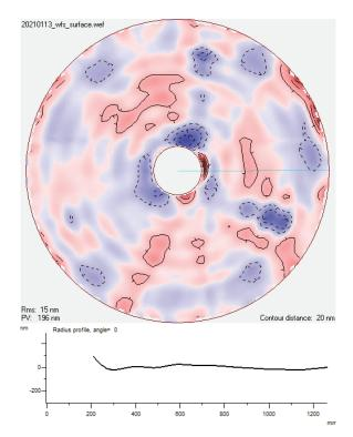
Figure 7. Latest surface accuracy measurement performed at OPTEON.
