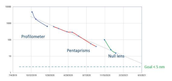
Log RMS for the shape accuracy of the optical surface of the mirror vs time
