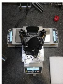
Figure 13: Derotator (STM) mass properties measurement.
