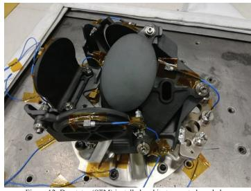
Figure 12: Derotator (STM) installed and instrumented on shaker table.
