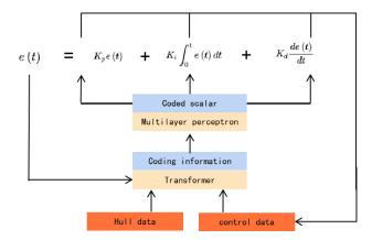
Figure 5. Dynamic PID parameter control method based on Transformer and MLP.
