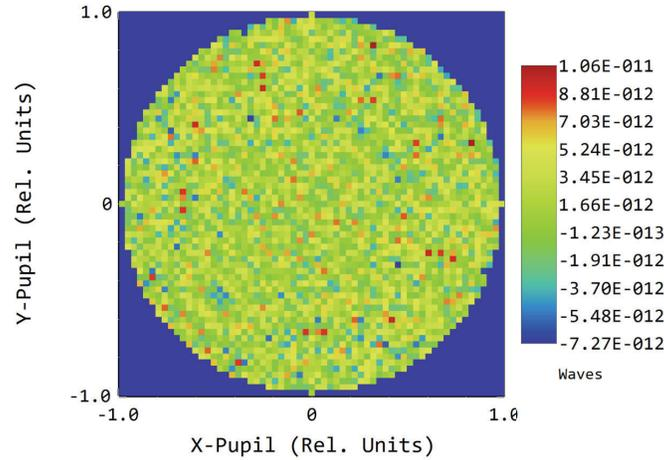
Figure 4. Wavefront map at the output of the axicon pair (wavelength = 1075 nm)
