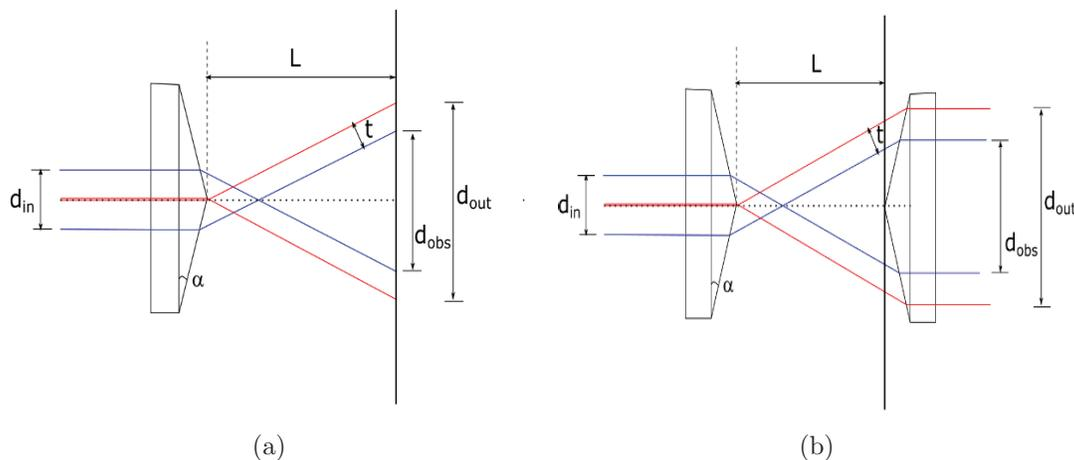
Figure 1. Schematic of the single axicon (a) and the axicon pair (b)
