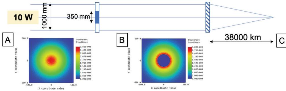
Figure 7. Physical optics propagation of an obstructed gaussian beam to a distance of 38000 km.
