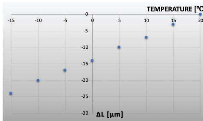
Figure 5. Thermal effects on the spacing between axicons (L) with Aluminium 6061 housing ( $CTE = 23.5 \times 10^{-6}/^{\circ}C$ ).
