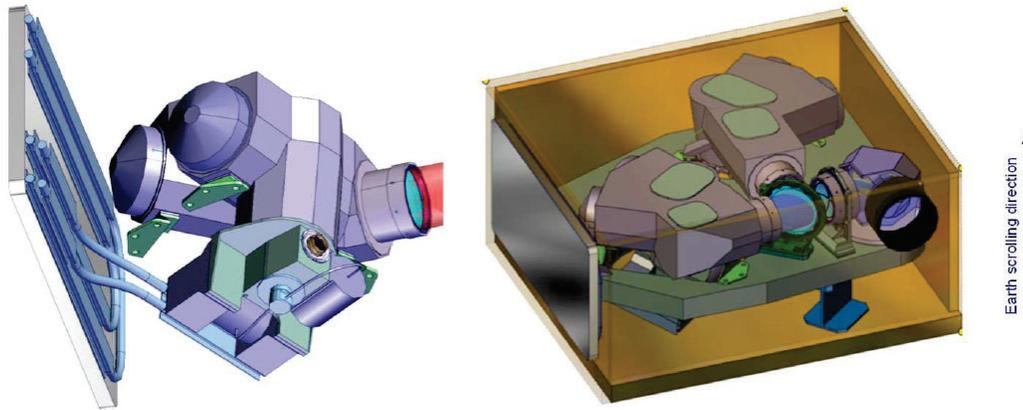
Figure 4. (Left) Bottom view of the EFP assembly for the SWIR channel, with the MCT detector unit visible at the bottom, connected to the radiator for the cryocooler. (Right) Top view of the Carbon-CGI payload, comprehensive of scanning mechanism (on the right) and two EFP assemblies for SWIR (leftmost) and VNIR (topmost).
