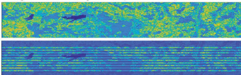
Figure 3. Example of classical image (top), and image detected by a CGI instrument, with modulation introduced by the variable OPD. Satellite velocity is in the vertical direction. The image is an albedo map at 760 nm from Sentinel-3 data.
