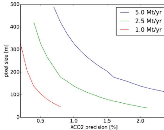
Figure 1. Relation between the minimum resolution (here pixel size) and XCO<sub>2</sub> precision required to estimate with 15% uncertainty the flux of a point source. The different line indicate difference flux levels.
