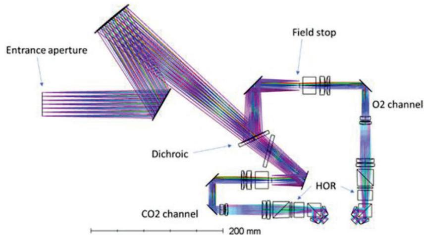
Figure 2. Concept optical design of the Carbon-HIGS instrument, comprehensive of the common front telescope and two HIGS interferometers.
