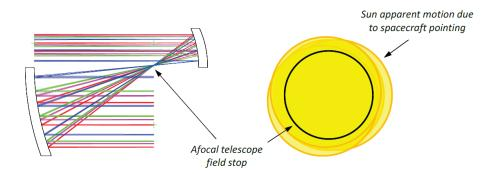
Figure 3: Implementation of afocal array field stop.
