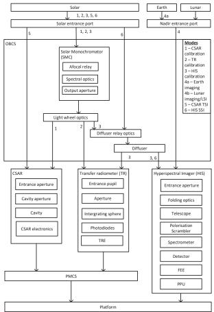
Figure 2: Payload optical and electrical signal chains
