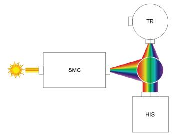
4. Calibration of the HIS gain through processing of the preceding measurement data.
