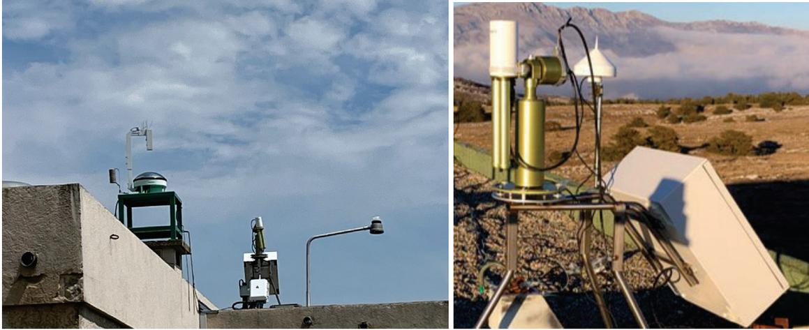
Figure 8. The Cimel CE318-T photometer installed near the Réuniwatt camera on the roof of the MéO station at Calern Observatory.
