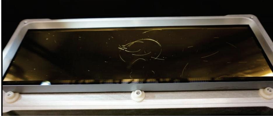
Figure 7. Final visual inspection of the gold coated NIRPS grating before delivery.
