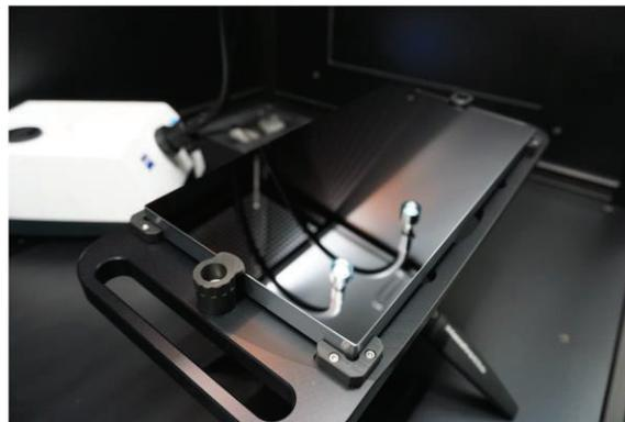
Figure 4. Silicon substrate at visual incoming inspection before start of grating manufacturing.
