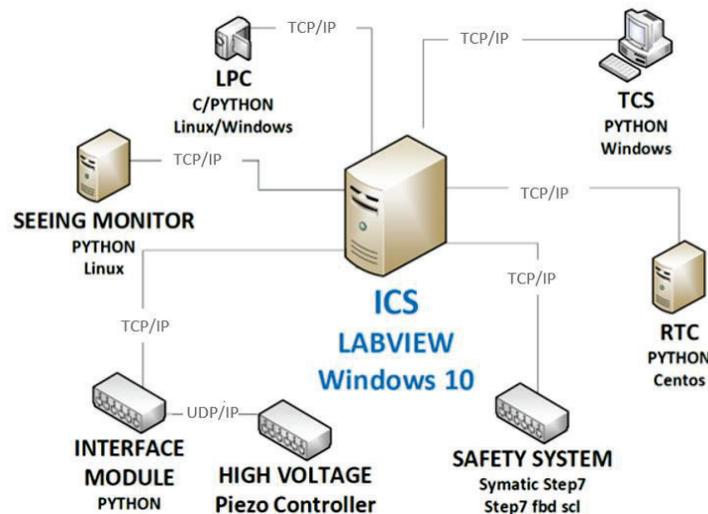
Figure 10. A schematic of the ICS with server software communication among different units.
