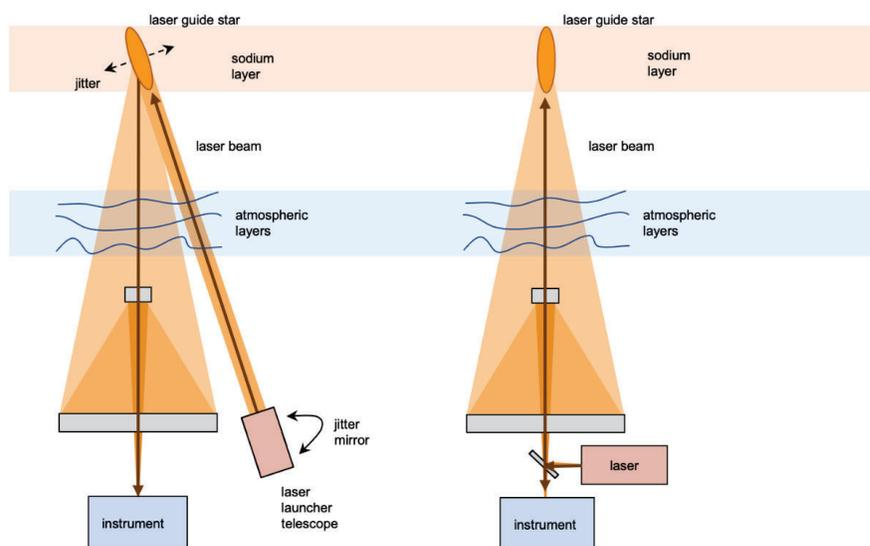
Figure 13. Bistatic (left) and Monostatic (right) propagation schemes. The uplink laser beam can be corrected (pre-compensated) in monostatic mode, since the downlink and uplink atmospheric volumes are the same, for the wavefront sampled by the Py-WFS. Note that the WFS and the uplink corrections do not suffer from cone effects (focal anisoplanatism)
