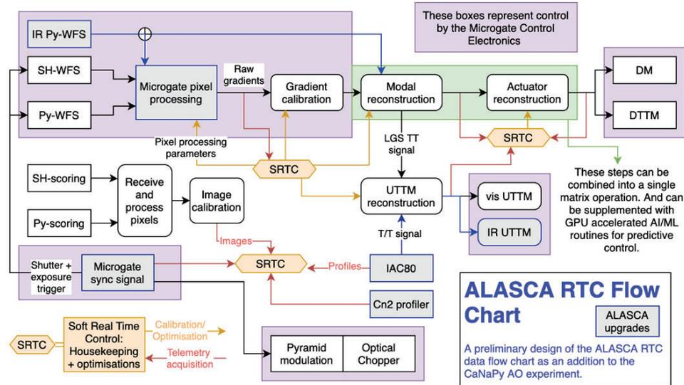
Figure 11. The main high-level view of the data flow in the system RTC. The core loop software is derived from the Durham Adaptive-optics Real-time Controller (DARC), modified and adapted.
