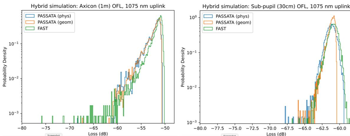
Figure 17. Histogram plots showing the distribution of power received by the ALPHASAT GEO satellite (as a fraction of transmitted power in dB) at 38000 km from Earth, when closed loop LGS-AO is used for the OFL uplink pre-compensation. The two plots correspond to nighttime configuration (left, 1.016m diameter pupil) and daytime (right, 0.30m pupil) launch geometries, monostatic propagation
