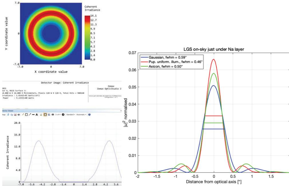
Figure 14. Left: laser beam intensity distribution at the OGS 1.016 m diameter primary mirror after conversion of the Gaussian beam into a Laguerre-Gauss annular beam, using double-axicon optics. Right: PSF of the LGS at 90 km, without turbulence, for the three cases described in the text
