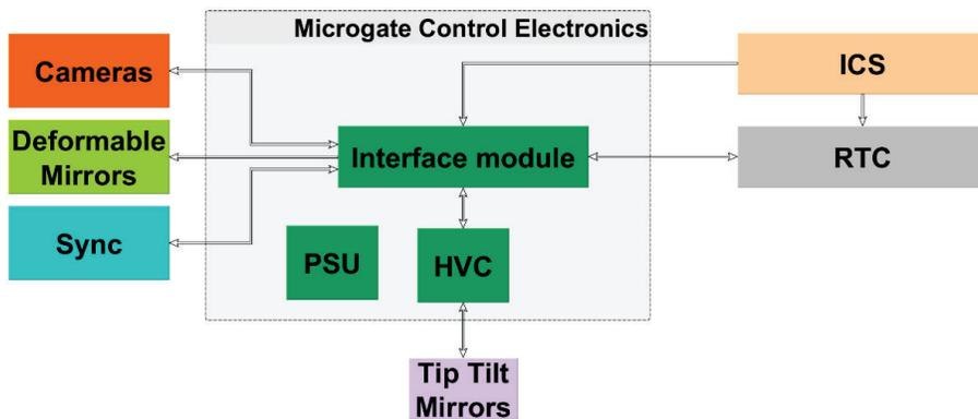
Figure 12. ALASCA control system layout. HVC, High Voltage Control, is a dedicated digital fast piezo mirror control already produced by Microgate, controlling the tip-tilt mirrors. The Interface module (IM) interconnect the hardware on the bench with the RTC, merging sensor data, synchronizing of the sensors' frames, distributing the mirror commands and configuring sensors and mirrors parameters
