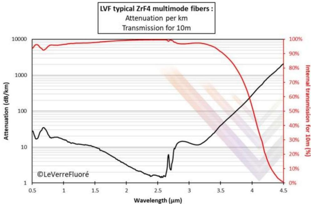
Figure 4 Transmission for a ZrF<sub>4</sub> Fiber
