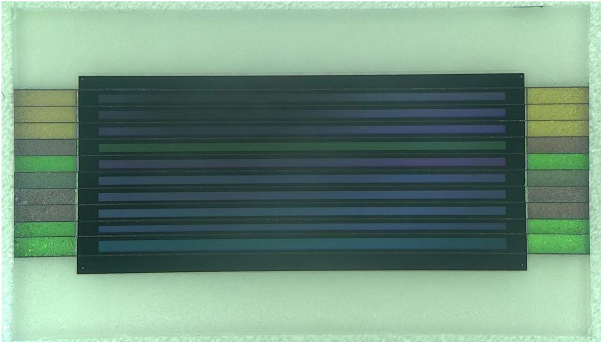
Figure 14 multispectral filter with aperture mask and outer edge unmasked (the individual filter bars and the glue gaps between them can be nicely seen).
