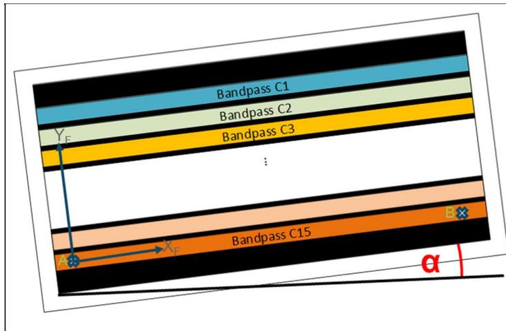
Figure 10 Coordinate system of the filter. The translation stage coordinates (not shown) were assumed to be exactly horizontal and vertical in the image. The clocking angle  $\alpha$  is determined with the setup can be compensated for each measurement spot.
