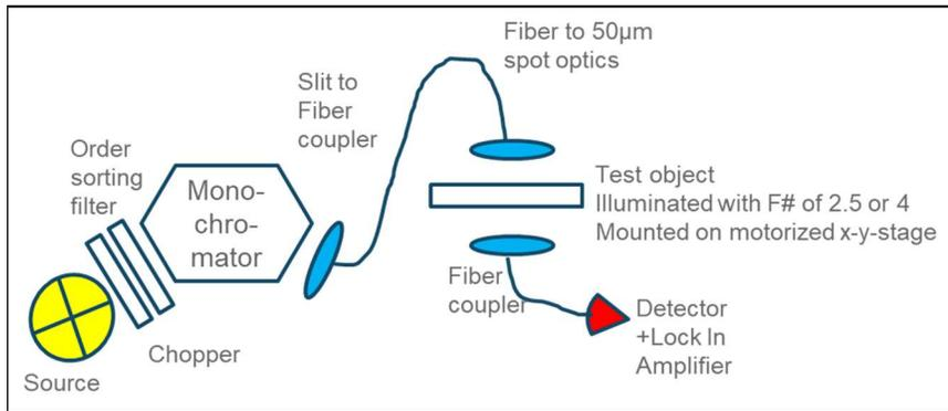
Figure 2 conceptual layout of the spectroscopic setup
