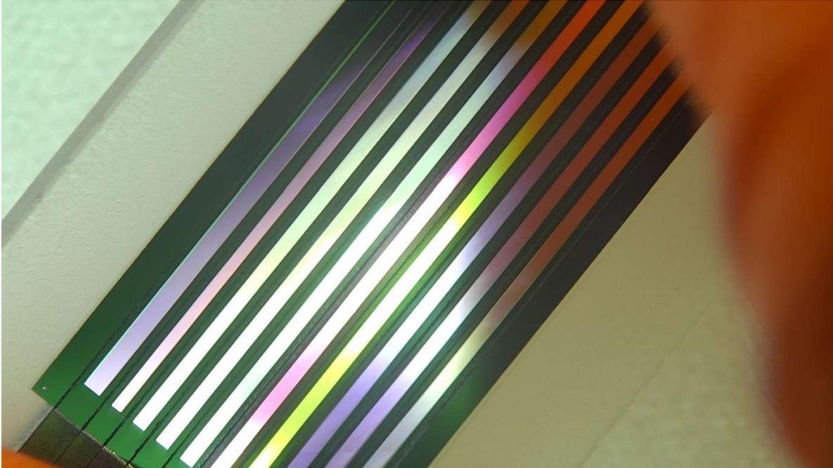
Figure 13 multispectral filter in visual inspection: glue gaps are visible as thin dark stripes, covered by the aperture mask of the filter.
