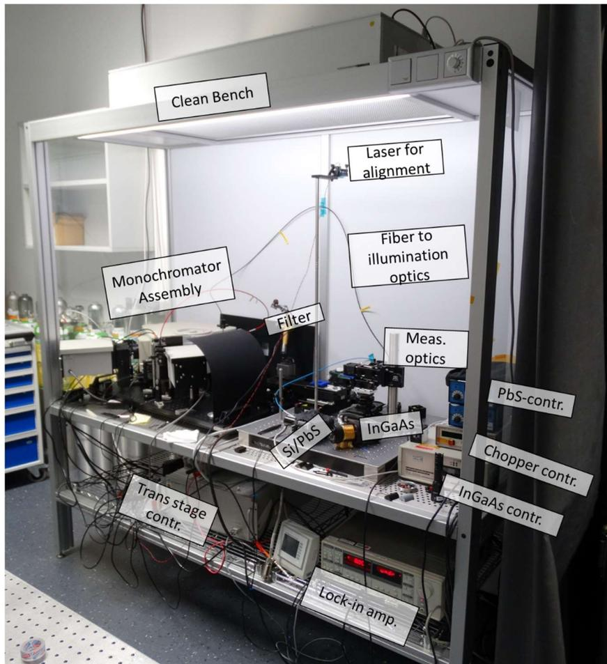
Figure 3 Metrology setup at optics LAB at OHB Munich
