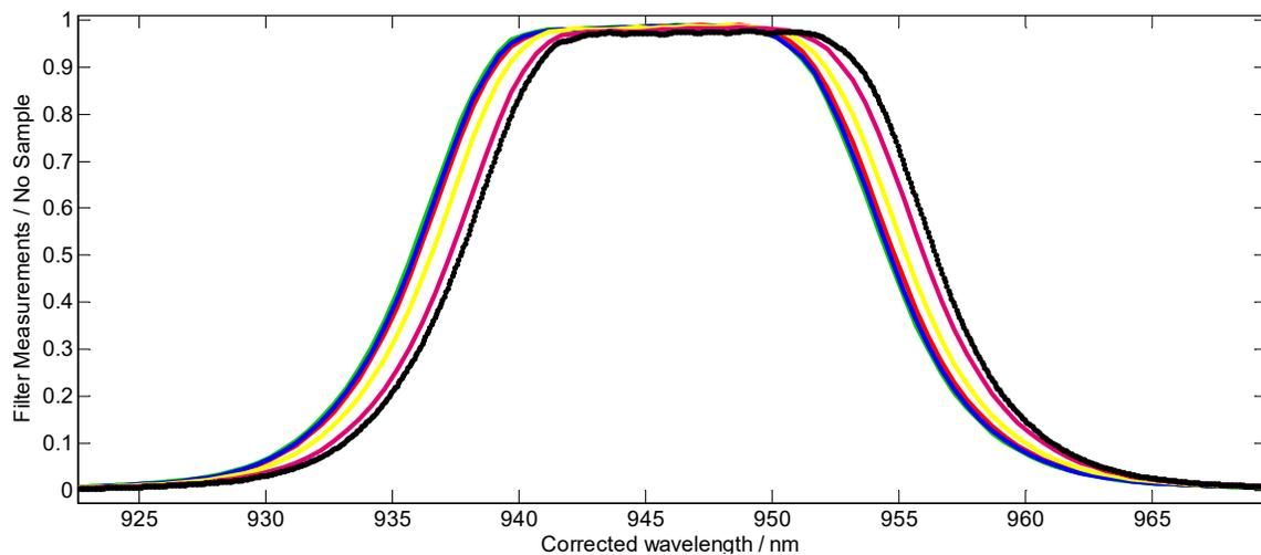
Figure 16: Band 1: The first 3 positions lie close together; there is a clearly visible inhomogeneity. Still the transmissions are well within the requirement.
