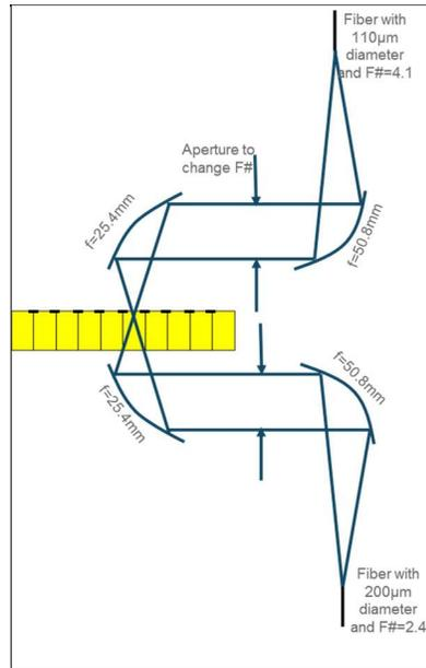
Figure 5 Optical path of the transmission optics with filter functional surface in the intermediate focus. The dark sections on the filter upper surface indicate the aperture mask, which separates the individual spectral channels and covers the glue gap between the individual filter bars.
