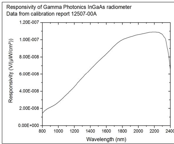
Figure 9 Responsivity of the Gamma photonics InGaAs radiometer
