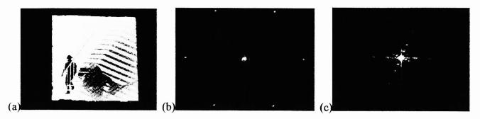
Fig.10. (a) Scene; (b) Diffraction pattern; (c) Magnified diffraction pattern.
