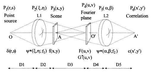
Fig.1. Geometry of the optical convergent correlator.  $L_1$  and  $L_2$  are convergent lenses. O' is the image of O given by  $L_1$ , and A' is the image of A given by  $L_2$ .
