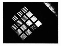
Fig.5. Tilted gratings with respect to the pixel ordering in the CCD camera.
