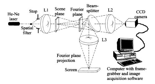
Fig.2. Experimental set-up: convergent optical correlator with two arms.
