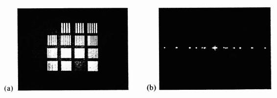
Fig.3. (a) Collection of diffraction gratings with different frequencies; (b) Fourier spectrum.
