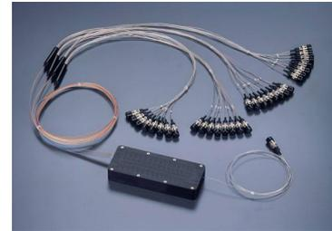
Fig. 3(b) AWG multi/demultiplexer
