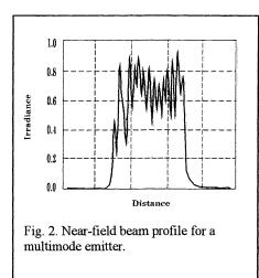
rolloff overlaid with some rippling effects, for a combination of both macroand micro- spatial non-uniformities. Thus, in the array direction, the emitters approximate miniature incoherent or partially coherent extended sources. Furthermore, as the emitters are generally not phase coupled with one another, the light from the various emitters can be superimposed at the modulator without incurring interference effects.
