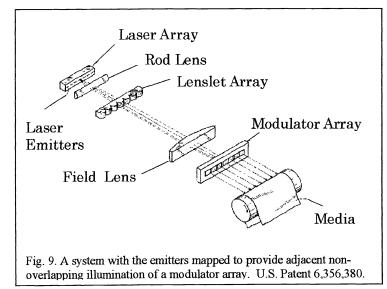
mapped (either far-field projections or near-field images) to the modulator array with each emitter illuminating one of a series of adjacent regions of the modulator array. In the cross-array direction, the rod lens works with other optical elements, to image the beams directly to the modulator array. The modulator array is, in turn, imaged to the media by a printing lens (not shown).
