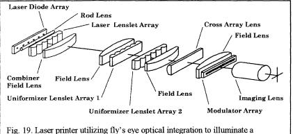
direction, the fly's eye integrator telecentrically flood illuminates the spatial-light modulator arrav uniform light, while the cross array light is focused to form a beam waist at the modulator. In combination. anamorphic array and cross-array optics illuminate the modulator array with a long, narrow, line of light of uniform
