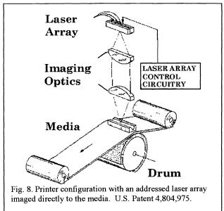
array of individually addressable laser diodes is monolithically integrated on a semiconductor substrate. The system uses spherical optics to image the laser array directly onto the media, so each laser diode corresponds to a pixel in a line on the print. While a variable response from laser emitter to laser emitter across the laser array can potentially be corrected via a calibration process, any outright emitter failures would provide uncorrectable line artifacts.
