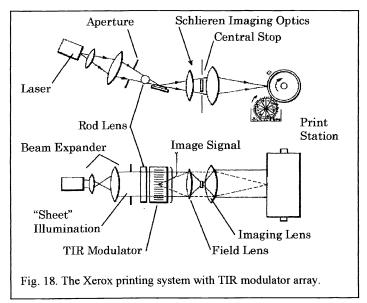
array direction onto the modulator array. A threeelement anamorphic optical system was used in the cross-array direction to focus the light to the modulator array. In the case that a Gaussian beam laser source was used,<sup>41</sup> the illumination system could be equipped with an apodizer to make uniform the array-direction spatial-light profile to within a few percent but at the cost of a 50% light loss.
