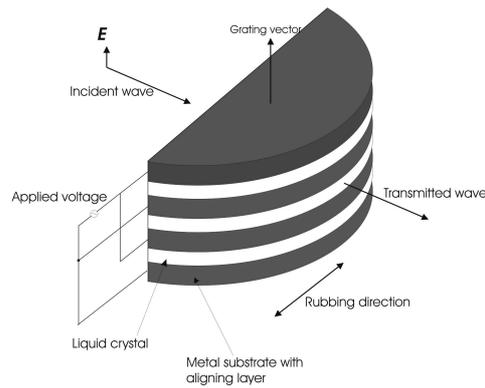
Figure 2. Liquid crystal microwave lens fabricated by Tanaka and Sato<sup>6</sup>.
