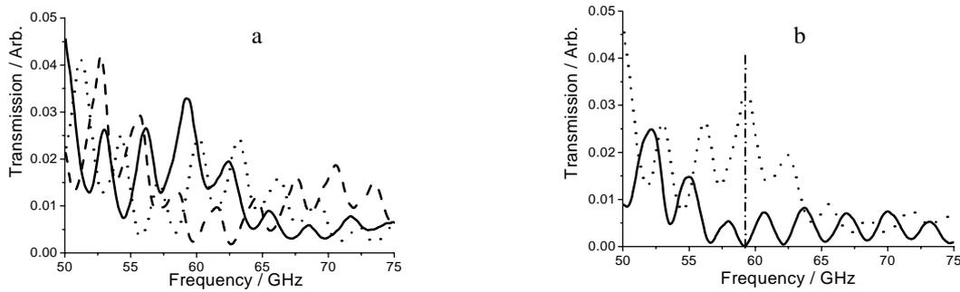
Figure 9. Transmission data as a function of frequency for different voltages applied to all cells. a. The solid line is for no voltage applied, the dotted line is for a voltage of 1.6 V<sub>rms</sub> and the dashed line is for a voltage of 3.0 V<sub>rms</sub>. b. The dotted line is for no voltage applied and the solid line is for the top six gaps in each group of ten having applied voltages of 3.0 V<sub>rms</sub> with the remaining four gaps having applied voltages of 1.6 V<sub>rms</sub>.
