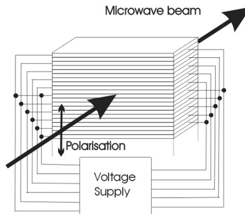
Figure 8. Part of a stack of liquid crystal filled metal slits which comprise a voltage-tuned microwave beam steering device<sup>21</sup>.
