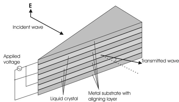
Figure 1. Geometry used by Tanaka and Sato<sup>4</sup> for the liquid crystal prism device.
