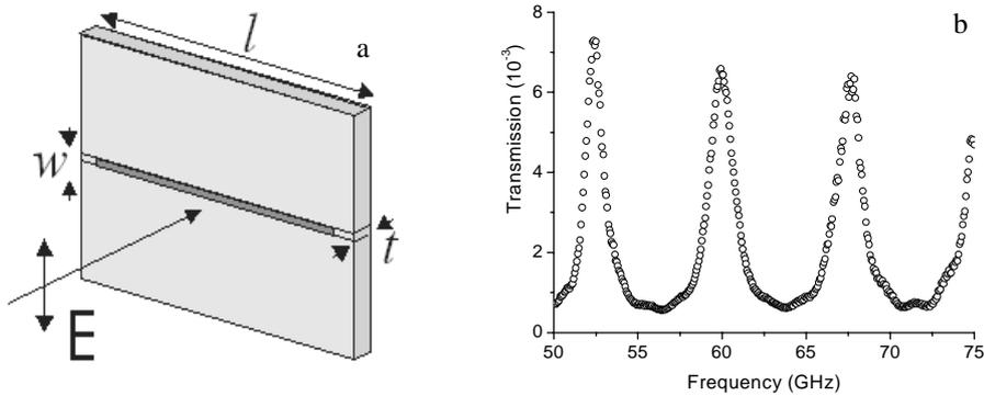
Figure 4. a. Geometry to be explored for resonant transmission of a single variable width slit in an aluminium plate of thickness  $t$ . The microwave field is polarised orthogonal to the slit and incident normally on to the metal plate. b. Typical transmissivity scan for a slit width of  $250\ \mu\text{m}$ .
