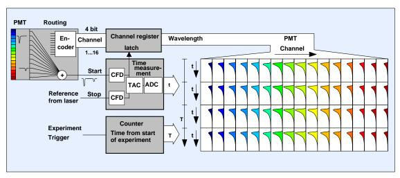
Fig. 4: Sequential recording
