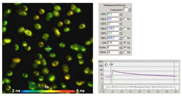
Fig. 10: Lifetime image built up in the time-tag mode. Amplitude-weighed lifetime of triple-exponential decay. Spores of amanita citrina, 512x512 pixels, 256 time channels, Becker & Hickl DCS-120 scanner and SPC-150 TCSPC module
