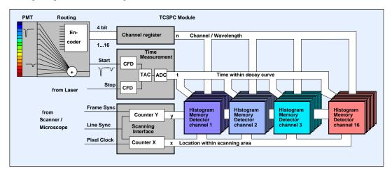
Fig. 7: Combination of multi-dimensional TCSPC with scanning
