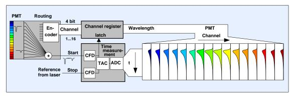
Fig. 2: Multi-wavelength TCSPC
