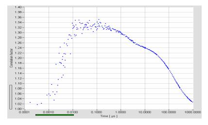
Fig. 11: Fluorescence correlation of a Rhodamin 110 solution over a range from 100 ps to 1 ms. Becker & Hickl DPC-230 TCSPC / Correlator board.
