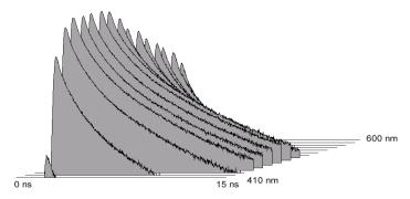
Fig. 3: Fluorescence of human skin, measured by multi-wavelength TCSPC. Excitation wavelength 405 nm, excitation power 60  $\mu$ W, acquisition time 5 s.
