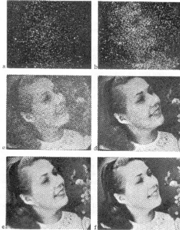
Fig. 5. Would a rose with fewer quanta smell so sweet? Pictures made with an increasing number  $N$  of photons: a.  $3 \times 10^3$ , b.  $1.2 \times 10^4$ , c.  $9.3 \times 10^4$ , d.  $7.6 \times 10^5$ , e.  $3.6 \times 10^6$ , f.  $2.8 \times 10^7$ . “The numbers of photons  $N$  refer to the total number of photons in the picture if the picture were uniformly at its high-light brightness,” per Rose [17].
