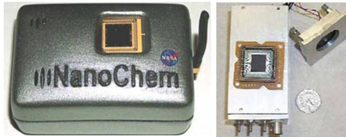
**Fig. 2.3-2** Complete NASA-Ames SWCNT sensor package
