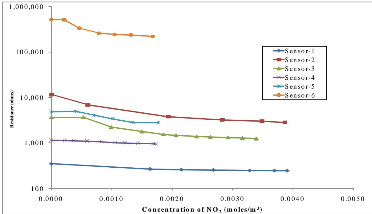
**Figure 3.1-2** Sensor Calibration Curves for NO<sub>2</sub> Detection
