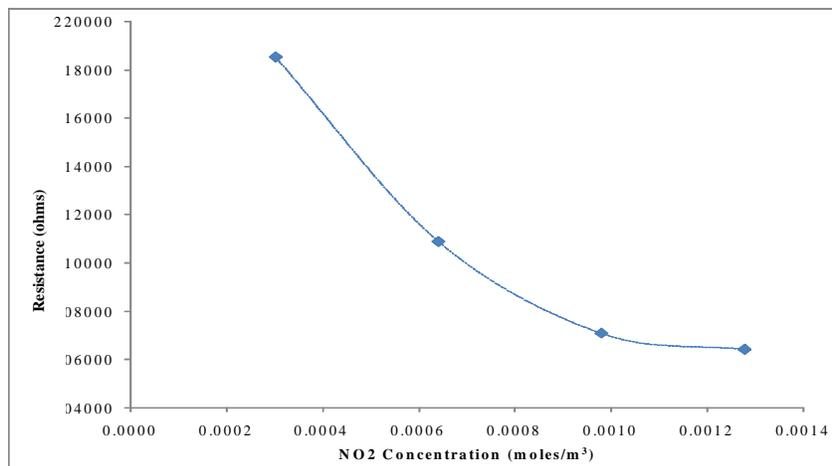
**Figure 3.2-2** Calibration Curve for Sensor in Aging Cup Configuration
