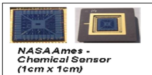
Fig. 2.0-1 Multi-channel sensor array (NASA-AMES)
