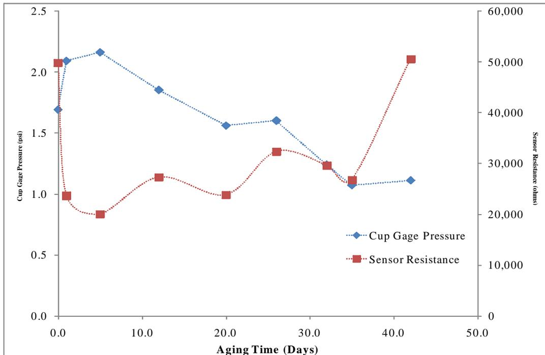
**Figure 3.2-3** Pressure and Sensor Data from Propellant Aging Experiment
