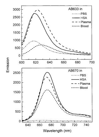
**Fig. 2** Relative emission spectra of 3  $\mu$ M AB633 (top) and 3  $\mu$ M AB670 (bottom) in PBS (----), 4 g/dl HSA (---), plasma (---), and whole blood (--). Front face geometry was used for measurements in HSA, plasma and blood.
