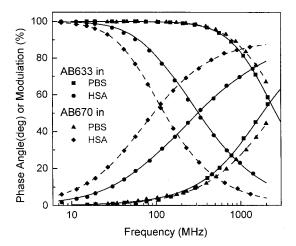
**Fig. 4** Phase angles and modulations of AB633 in PBS ( $\blacksquare$ ) and HSA ( $\bigcirc$ ), and AB670 also in PBS ( $\blacktriangle$ ) and HSA ( $\blacklozenge$ ). Excitation was at 600 nm, while observation was at 630 nm for AB633 and 670 nm for AB670. Dye concentrations was 3  $\mu$ M while HSA concentration was 200 mg/L.
