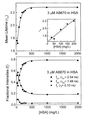
**Fig. 6** Variation of the mean lifetime ( $\bar{\tau}$ ) of 3  $\mu$ M AB670 (top) and corresponding fractional intensities ( $f_i$ ) (bottom) with different concentrations of HSA. The terms  $f_{b1}(\blacksquare)$  and  $f_{b2}(\bullet)$  represent the fraction intensities of bound AB670 while  $f_f(\blacktriangle)$  represents the fraction intensity of the free dye in solution.
