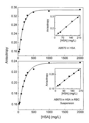
**Fig.** 7 Variation of the anisotropy of 3  $\mu$ M AB670 with HSA in PBS (top) and in 10% Hct red blood cell suspension (bottom). Insets show expanded HSA scale in the low concentration regions. Excitation was at 650 nm and observation at 678 nm.
