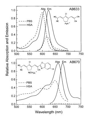
**Fig. 1** Relative absorption and emission spectra of 3  $\mu$ M AB633 (top) and 3  $\mu$ M AB670 (bottom) in PBS (--) and 100 mg/L HSA (--). Insets are the respective structures of the dyes.
