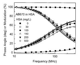
Fig. 5 Phase angle and modulation plots of 3  $\mu$ M AB670 in different concentrations of HSA. Excitation was at 600 nm and observation at 670 nm.
