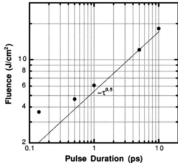
Fig. 7 Threshold fluence of water shock wave. The minimal fluence that causes surface-generated spherical shocks are defined as threshold. The solid line is fitted to the data and the slope is proportional to (pulse duration) $^{0.5}$ .
