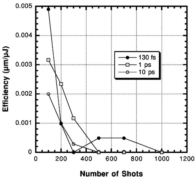
Fig. 6 Ablation efficiency defined by  $\mu\text{m}/\mu\text{J}$  is the highest for 130 fs pulses and decreases with longer pulse duration. Efficiency rapidly drops to near zero after several hundred shots.
