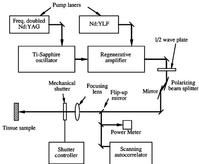
**Fig. 1** Experimental setup for hard tissue ablation. The pulse energy is controlled by rotating the  $\lambda/2$  wave plate. The energy per pulse and the pulse duration are measured by directing the beam to the power meter and to the autocorrelator. The mechanical shutter was used for allowing 1000 shots for each ablation craters. The repetition rate was 1 kHz and the beam size was 130 fs.
