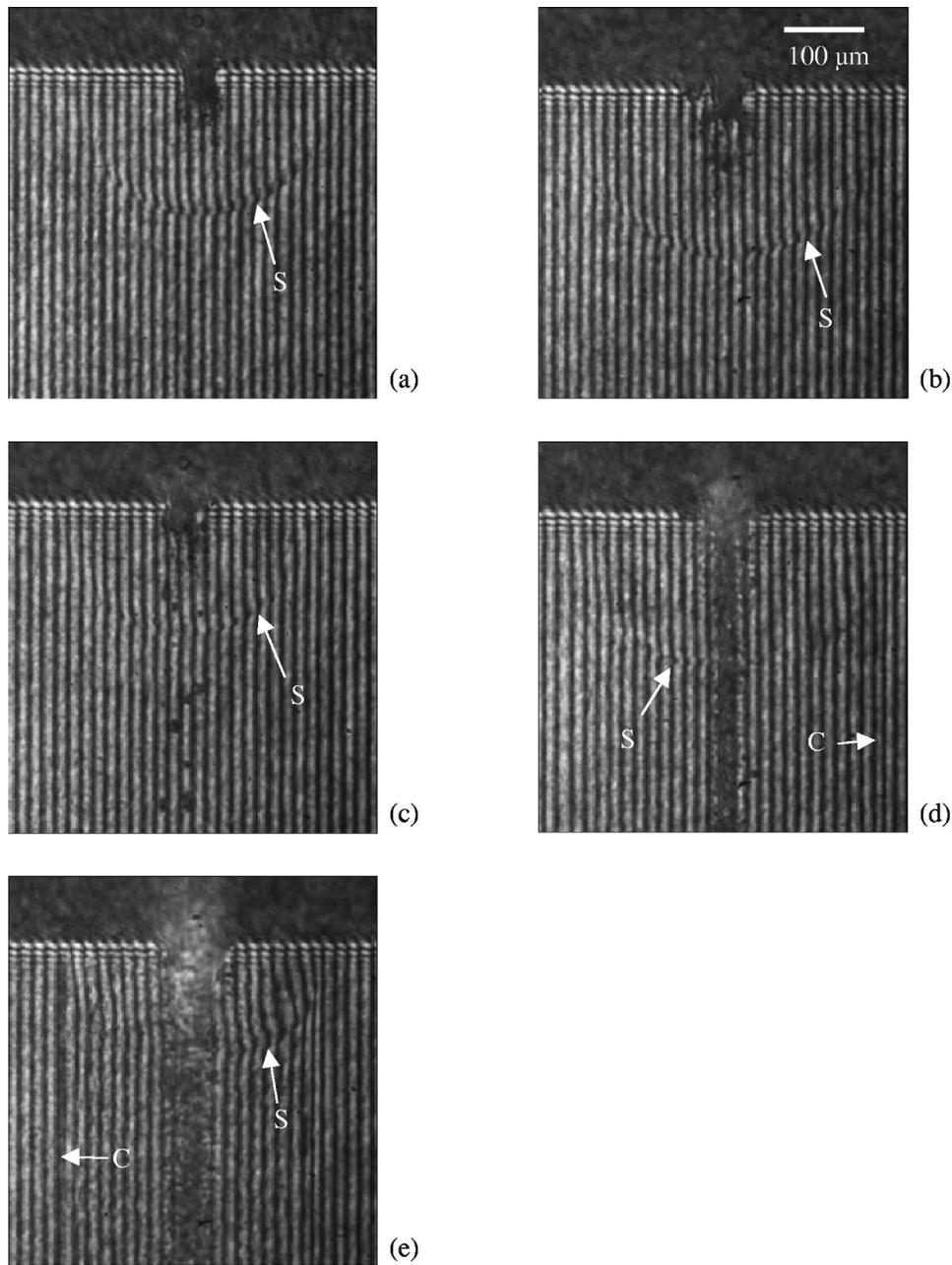
**Fig. 8** Interferograms of the USLP-induced shock waves. The pulse durations are: (a) 130 fs, (b) 500 fs, (c) 1 ps, (d) 5 ps, and (e) 10 ps. Cylindrical waves from beam axis are observed from the images of 5 and 10 ps (S: spherical wave, C: cylindrical wave).
