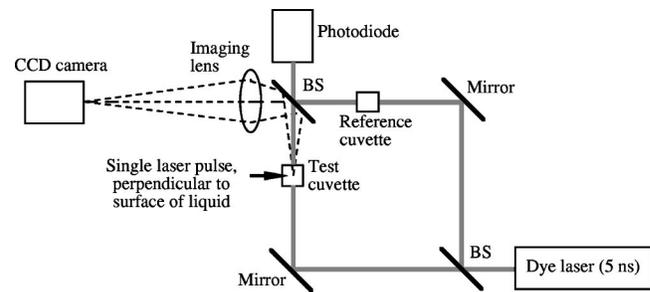
**Fig. 2** Mach-Zehnder interferometer for shock wave measurement due to USLP irradiation. The photodiode signal was used to control the time delay between USLP irradiation and probe beam. The USLP is incident vertically to the water surface inside the cuvette.
