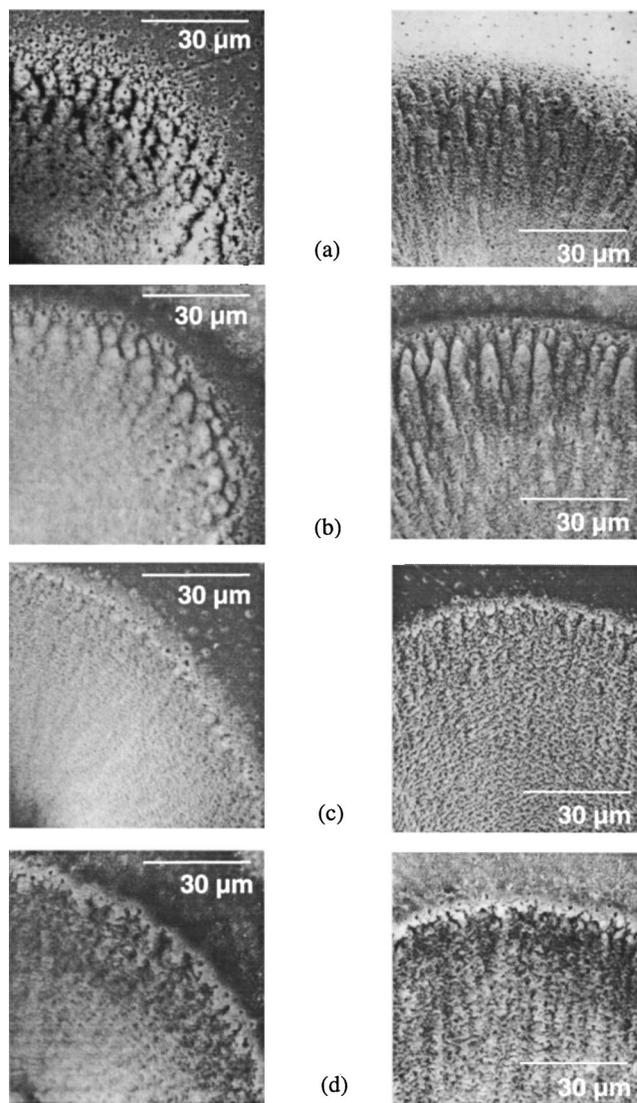
**Fig. 4** Top and side view of the ablation craters created by (a) 130 fs, (b) 1 ps, (c) 5 ps, and (d) 10 ps pulses. Two times the ablation threshold values (Figure 3) were used for each crater. It is observed that the edges of 5 and 10 ps craters melted indicating thermal accumulation. For 130 fs and 1 ps craters, the dentin tubules are open and intact both at wall and edge.
