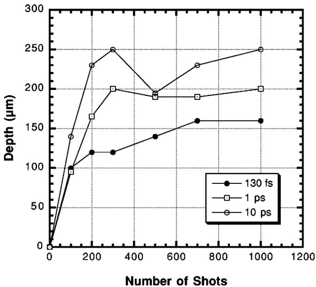
Fig. 5 Ablation depth as a function of number of USLP. Initial ablation rate is approximately  $1 \mu\text{m}/\text{pulse}$  for all cases. Longer pulse duration results in moderate improvement of final depth. Variations in ablation depth after 100–200 shots are mostly due to artifacts due to inhomogeneous materials.
