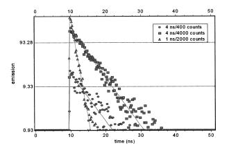
**Fig. 1** Simulated time-domain decay for 4-ns component (4000 counts), 4-ns component (400 counts), and a reference compound of 1 ns (2000 counts). The solid lines correspond to a fit using Globals WE software. The recovered lifetimes are reported in the text. The lamp curve (not shown) has a width of 300 ps.
