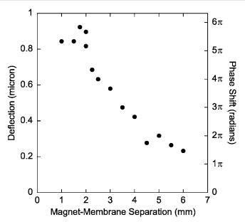
Fig. 3 Measured deflection of the flexible mirror and corresponding phase shift for the reflected optical beam.
