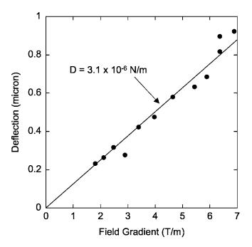
**Fig. 4** Membrane deflection versus the magnitude of the gradient of the applied magnetic inductance.
