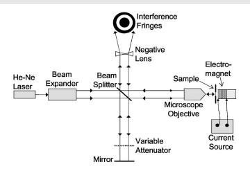
Fig. 2 Experimental setup for measuring the deflection of a flexible mirror in the field of an electromagnet.
