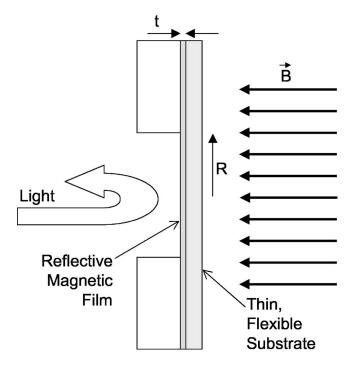
Fig. 1 Cross section of the flexible mirror, including Mylar® substrate and  $Fe_{0.55}Ni_{0.45}$  reflective magnetic film.
