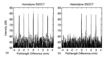
Fig. 3 Falloff measurements for (a) homodyne and (b) heterodyne SSOCTs acquired using setup in Fig. 1; the -3.5 dB signal falloff was preserved using heterodyne SSOCT; -60 dB calibrated reflector used in sample arm; 1 MHz heterodyne frequency shift.
