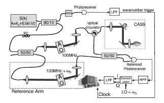
**Fig. 1** Heterodyne SSOCT system utilizing acousto-optic modulators. The swept-laser source has a center wavelength  $\lambda_0$ =1310 nm and bandwidth  $\Delta\lambda$ =100 nm. A balanced photoreceiver is used for dc artifact suppression. FFPI, fiber Fabry-Pérot interferometer; PC, polarization controllers; AO, acousto-optic modulator; C, circulator; CASS, anterior segment scanner.
