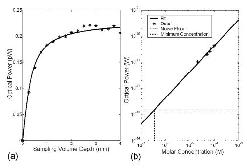
**Fig. 5** (a) Fluorescence signal power versus sampling volume depth: experiment ( $^*$ ), theoretical fit (solid line). Concentration of Rh:6G is 1  $\mu$ M. (b) Plot of the fluorescence signal power versus the fluorophore (Rh:6G) concentration: experiment ( $^*$ ), linear fitting (solid line), noise floor (dashed-dotted line).
