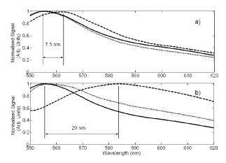
**Fig. 4** (a) Plot of Rh:6G fluorescence spectrum using bare fiber probe in clear solution (solid line), bare fiber probe in scattering phantom (dashed line), and DAFOS probe in scattering phantom (dotted line) and (b) plot of Rh:6G fluorescence spectrum using bare fiber probe in clear solution (solid line), bare fiber probe in fluorescent phantom (dashed line), and DAFOS probe in fluorescent phantom (dotted line).
