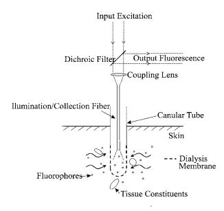
Fig. 1 Schematic diagram of DAFOS using a single fiber for illumination and collection.
