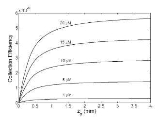
**Fig. 3** Theoretical fluorescence collection efficiency curves for a single fiber probe immersed in rhodamine:6G (Rh:6G), using molar concentrations in the range 1 to 20  $\mu$ M. The NA and core diameter of the fiber were 0.22 and 105  $\mu$ m, respectively; the refractive index of the sampling volume was 1.34; and the quantum efficiency ( $\eta$ ) was set to unity.
