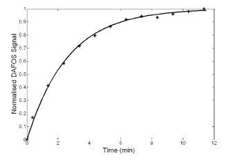
**Fig. 6** Plot of the normalized DAFOS signal versus time: experiment (\*), theoretical fitting curve (solid line).
